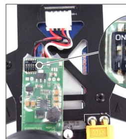
Dipswitch on the transmitter
